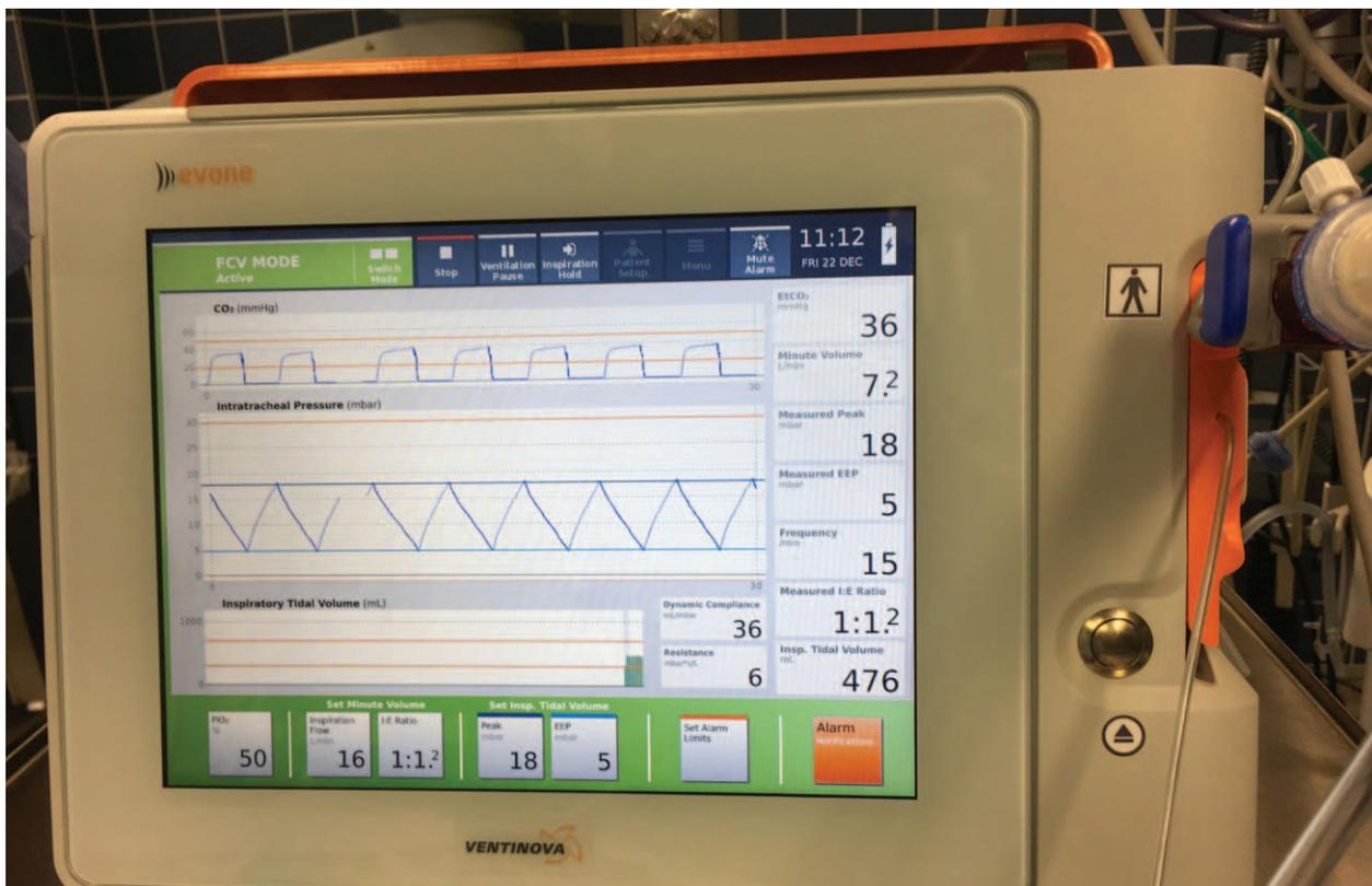
Photograph of the Evone ventilator (front), showing time course for mainstream capnography, tracheal pressure and inspiratory tidal volume. Adjustable settings are shown in the bottom of the screen. Measured variables appear on the right of the screen. On the far right of the housing, the orange-coloured cartridge (with the ejector inside), the attached sensor for mainstream capnography, the heat and moisture exchange filter and the line for tracheal pressure measurement are captured.
